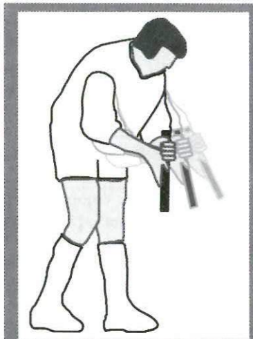
Looking down the tube, the floor should remain visible throughout the swing
