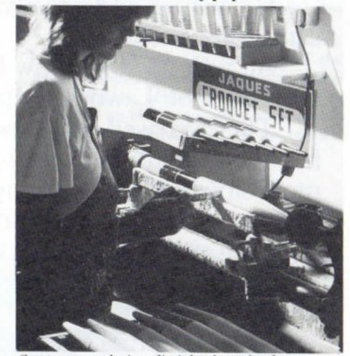
Centre pegs being finished at the factory
